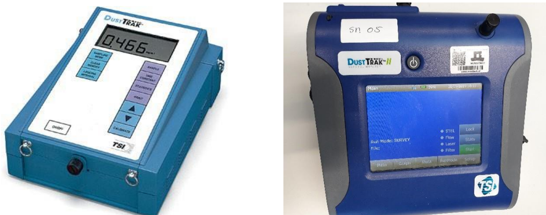
Figure 2.3 DustTrak models used for measuring PM 10 . Left model 8520, right model 8530.
