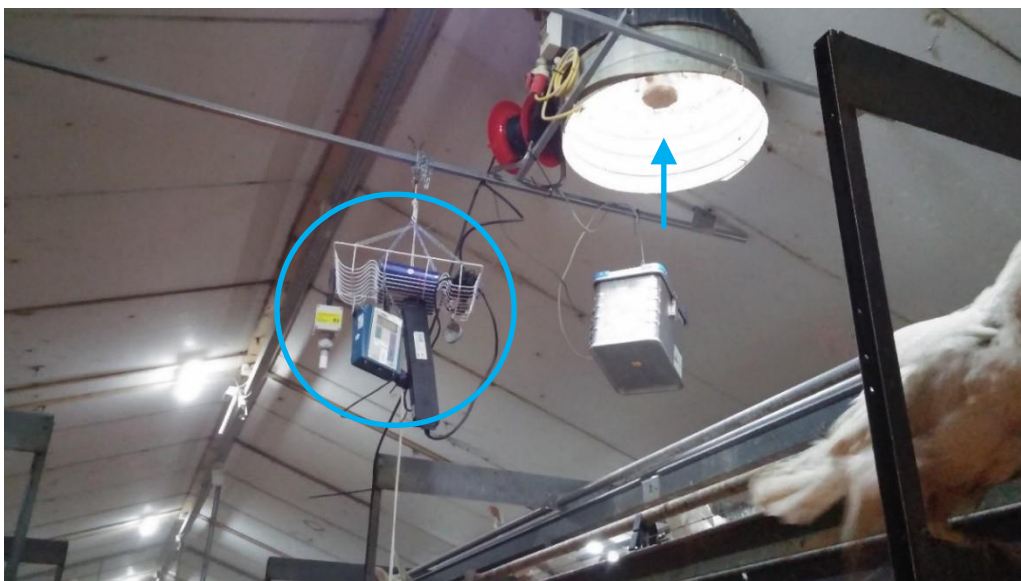
Figure 2.2 Location of the measurement of the concentrations in the house (circled in blue). The blue arrow indicates the air flow into the ventilation duct, outwards.
